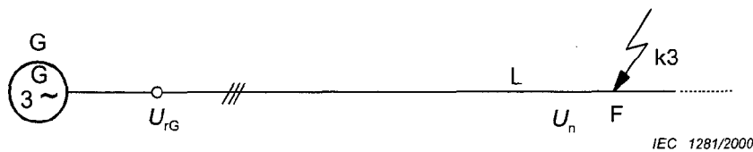
Figure 11b – Short circuit fed from one generator (without unit transformer)
